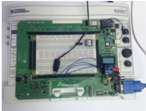
Figure 5. Xbee module mounted on the board NI ELVIS II +
