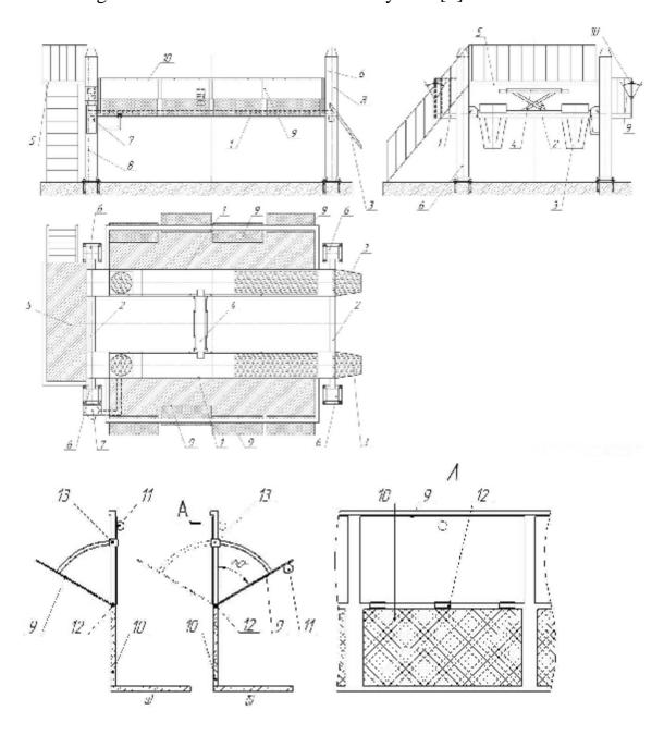
Figure 1 – The lift of balcony type for vehicles:
