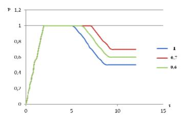
It is known that time of acceleration occupies less than 5 minutes from the beginning of movement. In the  $1^{st}$  picture the change of electric power of locomotive is shown at the beginning and after the acceleration movement. Also, a few variants of correlation of the power between the beginning and acceleration of movement and the electric power on the route (0.5, 0.6, and 0.7) are carried out on that picture.
